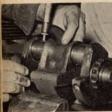
Crankshaft end-float should be 4 thou. If less, face off the white metal bearing by rubbing it on fine emery on flat plate
