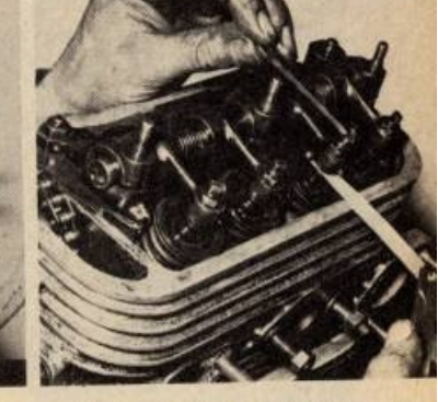
Valve clearances should be set when the engine is cold. On no account attempt this with a warm engine. Set to 18 thou
