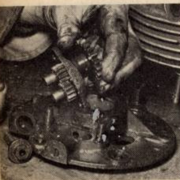
The oil pump gives no trouble. All that is necessary is to check balls for ridges, etc, and spring length against new ones
