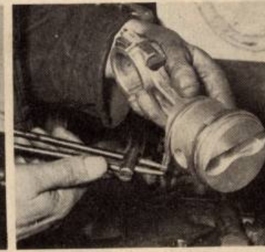
Small-ends never go as they have very little movement. The No. on con-rod must be on same side as highest edge of piston
