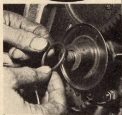
A rubber sealing ring goes on to shaft against the thrower plate. The half-time wheel is held by a circlip. Fit a new one
